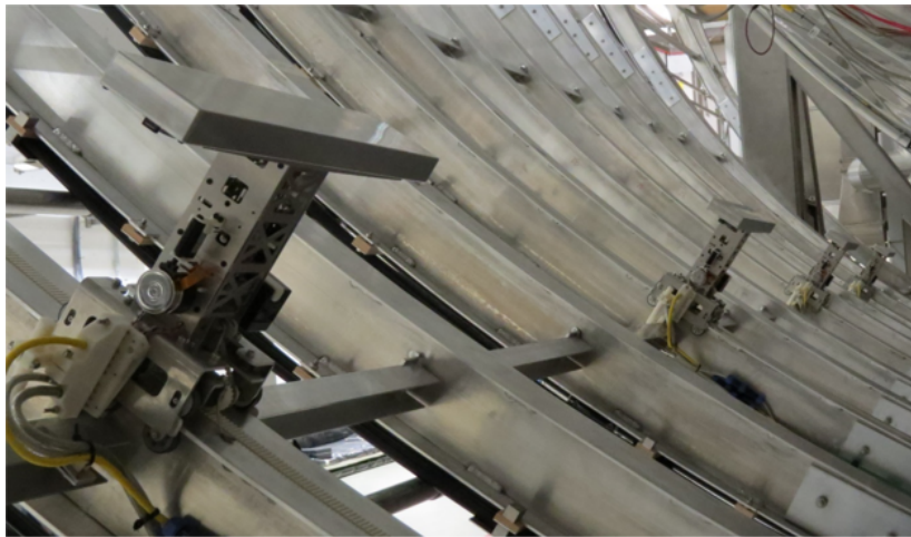
Figure 4: The four mounted mobile sensor units in their rest positions (docking stations) on the inner belts of the LFCS support structure. In the foreground the MobS unit on LFCS 3 close to the source side of the cylindrical part of the MS. Further away the MobS units on LFCS 6, 9 and 12 can be seen.
