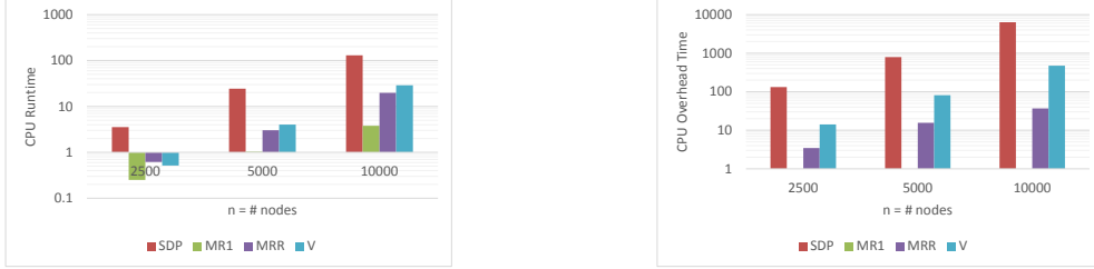
Figure 2: Top: CPU per-iteration runtime for four methods. Bottom: CPU runtime for overhead operations (rounding for SDP and MRR and initial matrix inversion or SVD for V). MR1 gives a vector output and has no additional overhead.
