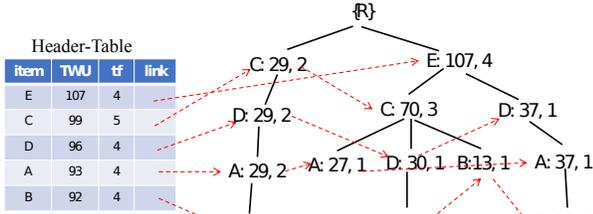
Fig. 3: Example  $IHUP_{TWU}$ -tree structure (used by IHUP [48]).
