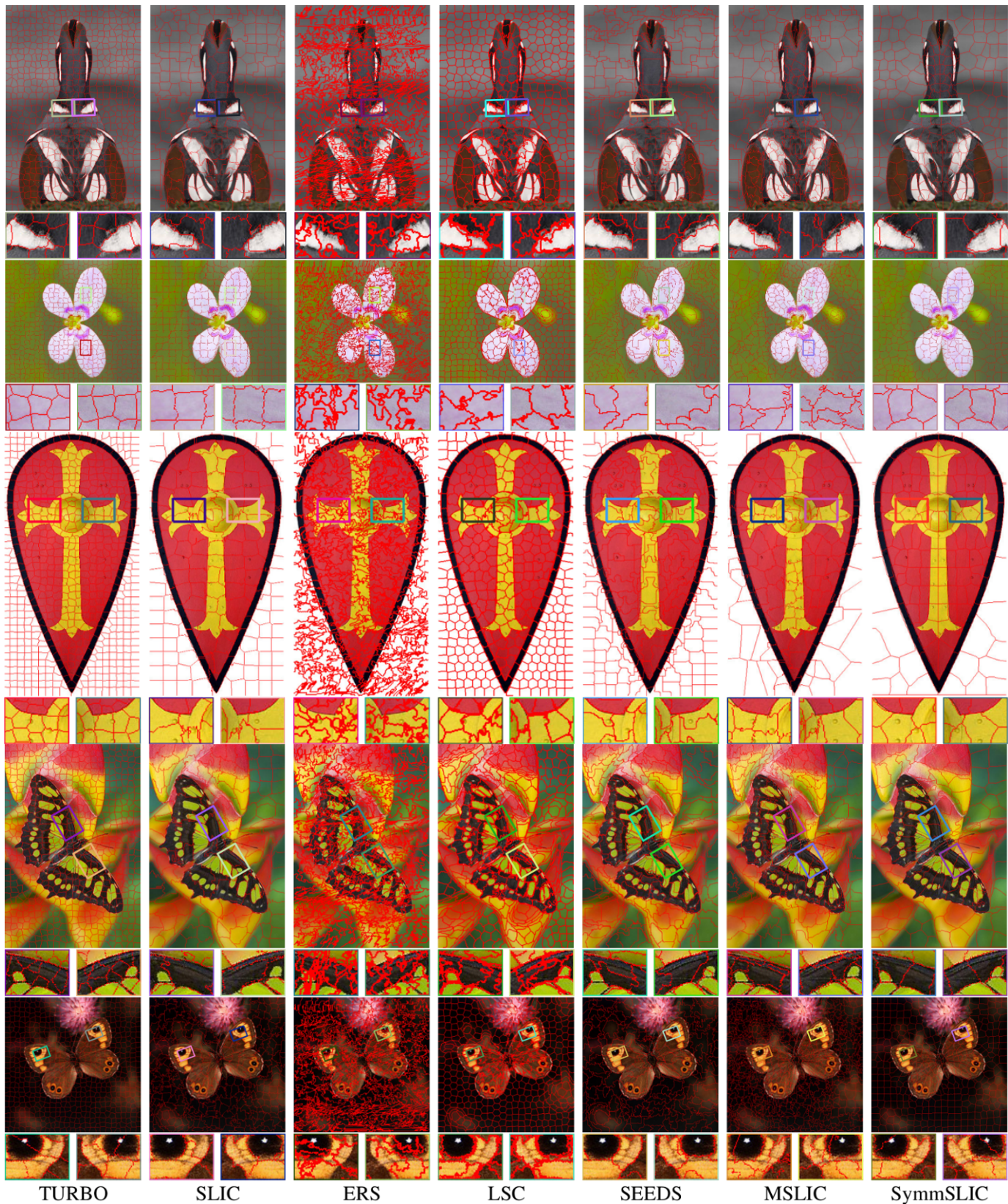
Fig. 10. Results for the approaches TURBO [27], SLIC [17], ERS [28], LSC [21], SEEDS [23], MSLIC [14], and the proposed method. For each image, we show two zoomed-in mirror symmetric windows to visualize whether the superpixels are mirror reflections of each other or not. Window border represents its location in the image. The tilted windows are aligned horizontally.
