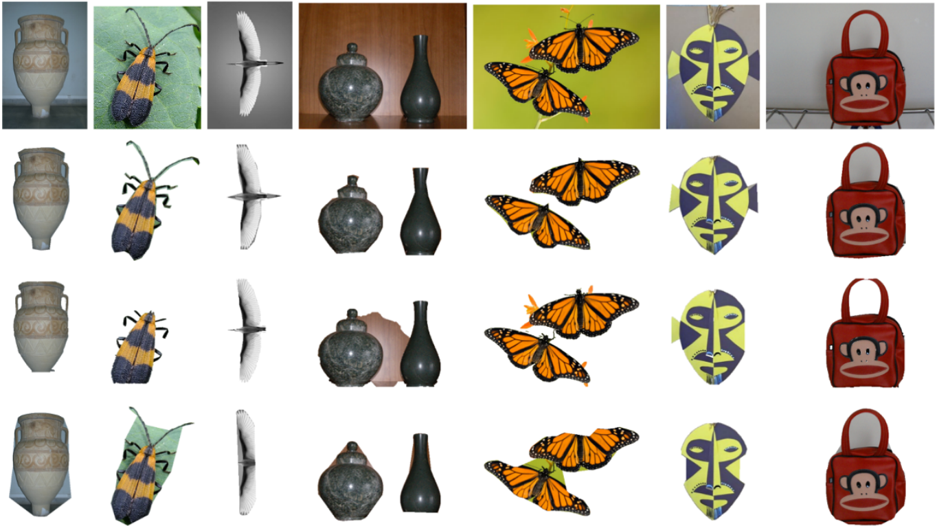
Fig. 9. Row 1: Input images, Row 2: the ground truth object segmentation, Row 3: grab cut in one cut [69] segmentation which requires a input mask around the object, and Row 4: unsupervised symmetric objects segmentation using proposed approach which does not require any input mask.
