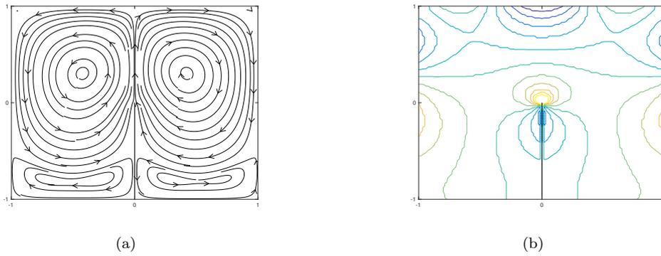
Figure 6: Streamline plot of the discrete eigenfunction  $\mathbf{u}_\ell$  (a), and plot of the discrete pressure  $p_\ell$  (b).
