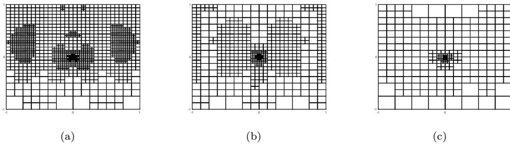
Figure 8: Adaptively refined meshes for  $RT_1 \times Q_1$  (a),  $RT_2 \times Q_2$  (b), and  $RT_3 \times Q_3$  (c).
