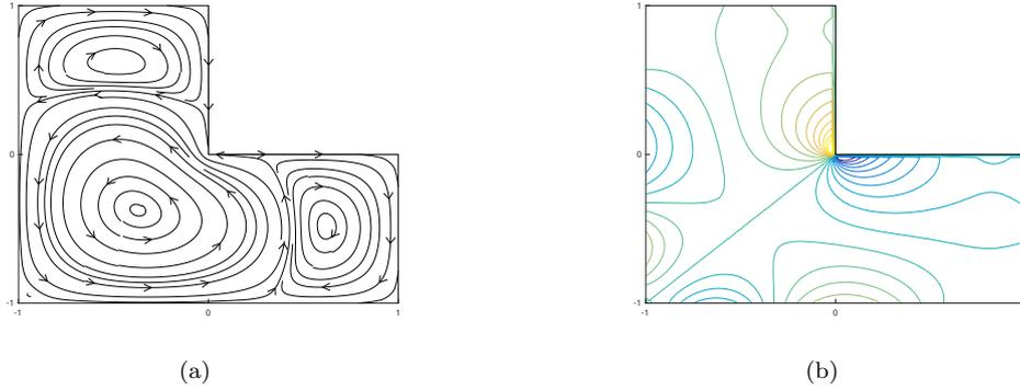
Figure 3: Streamline plot of the discrete eigenfunction  $\mathbf{u}_\ell$  (a), and plot of the discrete pressure  $p_\ell$  (b).
