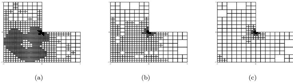
Figure 5: Adaptively refined meshes for  $RT_1 \times Q_1$  (a),  $RT_2 \times Q_2$  (b), and  $RT_3 \times Q_3$  (c).
