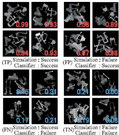
Fig. 7. Classification examples of the verification data. The numerical values indicate the estimated success rate by using the proposed CNN. The values in red indicate a successful picking classification, while the values in blue indicate a failure picking classification.
