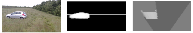
Fig. 6: Input image (left), classification based on semantic segmentation (middle) and corresponding ISM with detection cut-off after class occurrence along the focal axis
