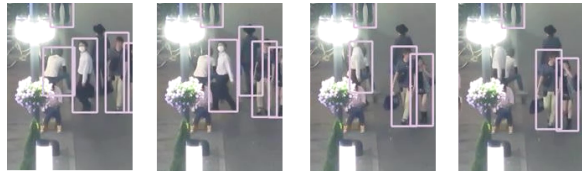
Fig. 7. Raw detections from MOT17 video 4, increasing in time from left to right. The leftmost person is occluded by someone who also becomes occluded.
