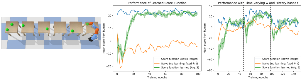
Figure 5: Domain 2 results. Left. A pybullet rendering of the task. The robot is a blue-and-orange arm, and each table is a zone. The green objects are spread across table surfaces. Middle+Right. See Figure 4 caption. Note. Learning curves are averaged over 5 independent trials, with standard deviations shaded in green.
