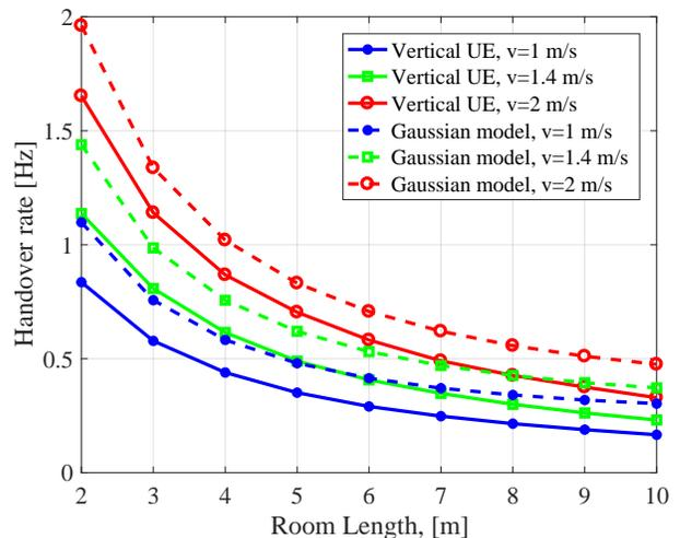
Fig. 7. Comparison of handover rate as a function of room length,  $L$ , for vertically upward UE and a UE with correlated Gaussian RP for  $\theta$ .
