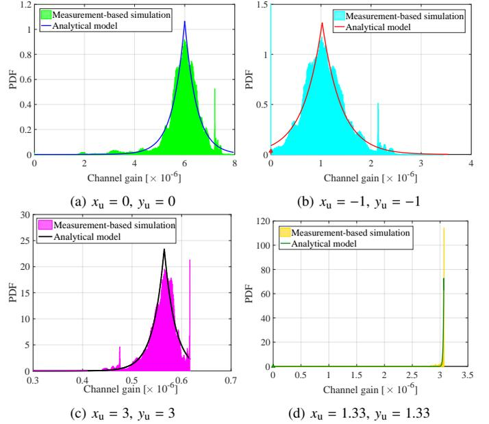
Fig. 5. Comparison between measurement-based simulations and analytical results of PDF of channel gain for different locations in the room with  $\Omega = \frac{\pi}{4}$ .
