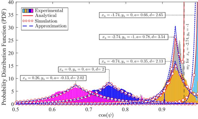
Fig. 4. Behavior of the sample PDF of experimental data and the closed-form PDFs with different locations of UE and fixed  $(x_a, y_a, z_a) = (0, 0, 2)$ ,  $z_u = 0$ ,  $\Omega = \pi$ , and for the sitting activity.
