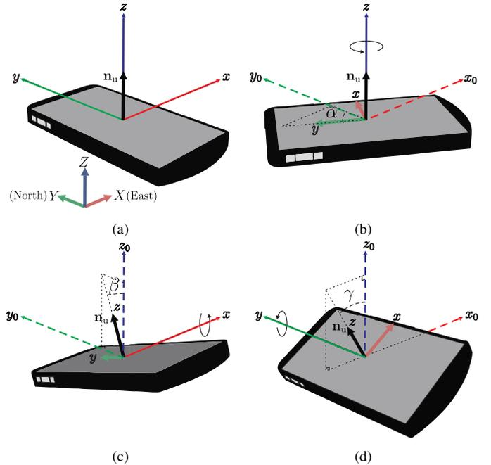
Fig. 1. Orientations of a mobile device: (a) normal position, (b) yaw rotation with angle  $\alpha$ , about the  $z$ -axis (c) pitch rotation with angle  $\beta$ , about the  $x$ -axis and (d) roll rotation with angle  $\gamma$ , about the  $y$ -axis.
