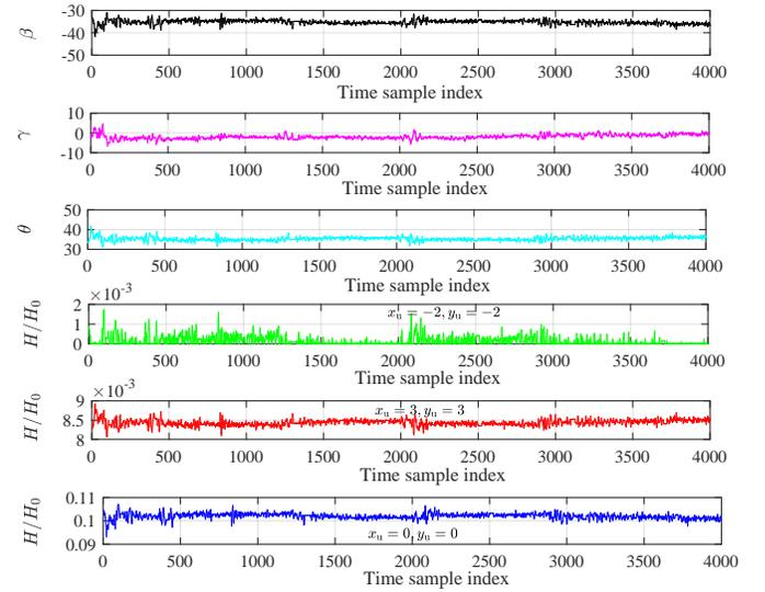
Fig. 6. Representation of one ensemble of the stochastic RPs,  $\beta$ ,  $\gamma$ ,  $\theta$  and the normalized LOS channel gain,  $H/H_0$ , for three UE's locations of  $(-2, -2)$ ,  $(3, 3)$  and  $(0, 0)$ . Here,  $\Omega = \frac{\pi}{4}$  and  $T_s = 13 \text{ ms}$ .
