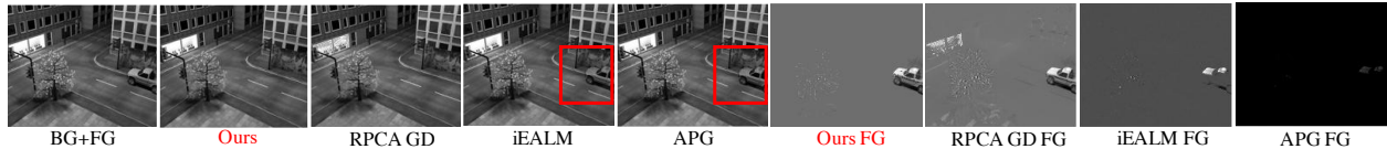
Figure 3: Background and foreground separation on Stuttgart dataset Basic video. Except RPCA GD and our method, all other methods fail to remove the static foreground object.
