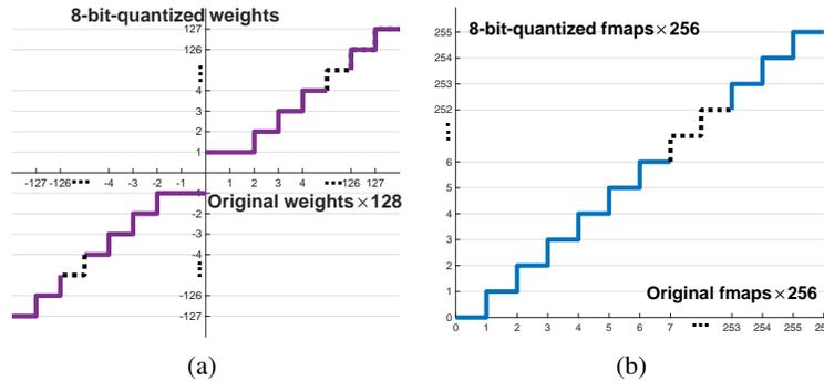
Figure 3: 8-bit quantization strategy of (a) weight and (b) feature map.
