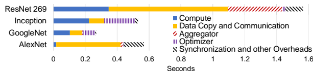
Figure 5: Progressive overhead breakdown of different stages during the distributed training pipeline for MXNet DDNN training on a 56Gbps network. Link capacity accounts for a small fraction of the copy and communication overhead in this setting.
