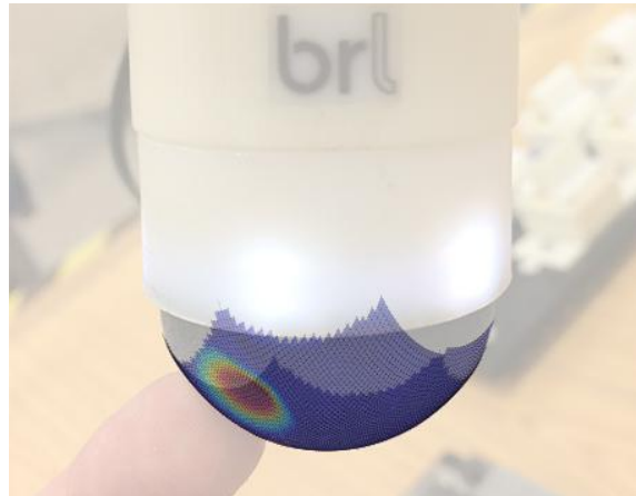
Fig. 1: The work presented here infers tactile features from TacTip sensory data by transducing a 3^{rd} dimension of the data via Voronoi tessellation. This data can be used to produce a 3D reconstruction of the sensor tip. Shown here is sensory snapshot, reconstructed and shown with the sensor.
