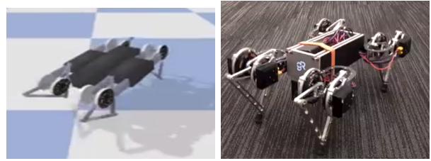
Fig. 1. Minitaur (from Ghost Robotics) executing a turning maneuver: in Bullet simulator (left), in reality (right), using our methods.
