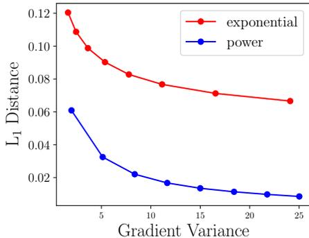
Figure 3: Average distance between  $\zeta$  and its binarized  $z$  vs. variance of  $\partial\zeta/\partial q$  measured on  $10^6$  samples from  $q(\zeta)$ . For a given gradient variance, power function smoothing provides a closer approximation to the binary variables.
