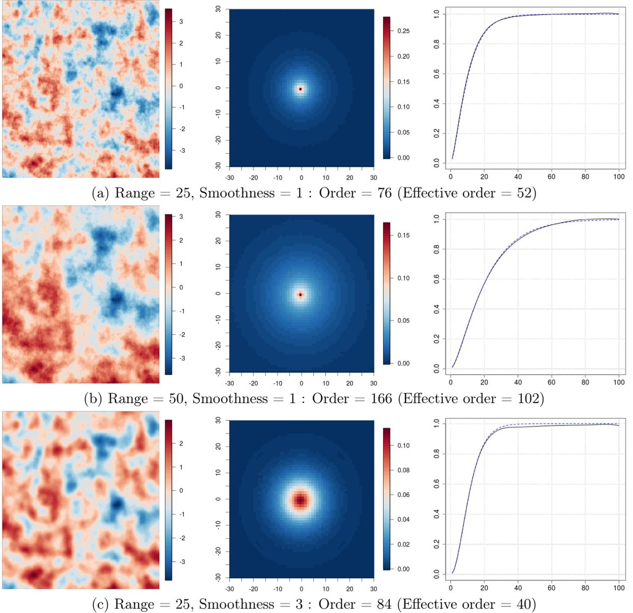
**FIG. 4 :** (*Left*) Simulations using Chebyshev approximation of a Matérn field on a 200x200 grid with various model parameters. (*Center*) Convolution kernels associated with the simulation. (*Right*) Mean variograms over 50 simulations (solid line) and model (dotted line).
