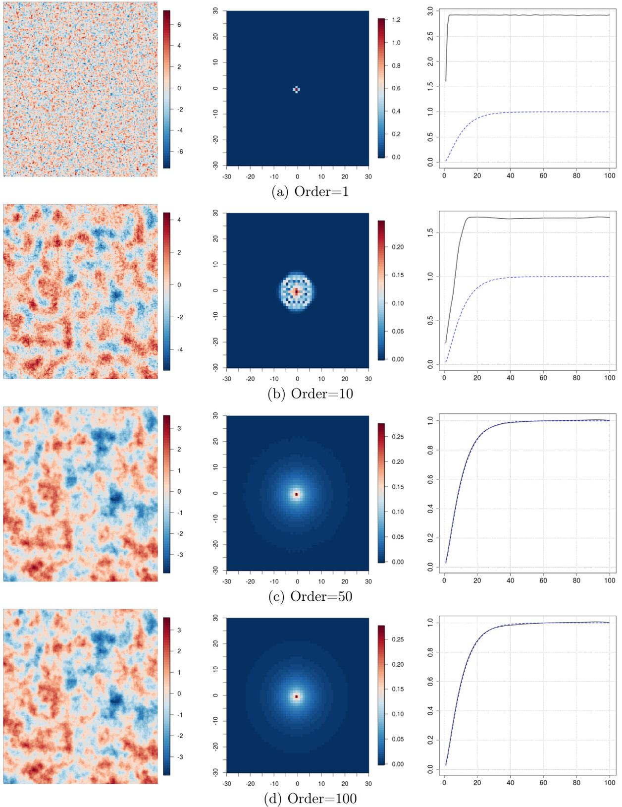
**FIG. 3 :** *(Left)* Simulations of a Matérn model with range 25, sill 1 and smoothness parameter 1 on a 200x200 grid using Chebyshev approximation with growing order. *(Center)* Convolution kernels associated with the simulation. *(Right)* Mean variograms over 50 simulations (solid line) and model (dotted line).
