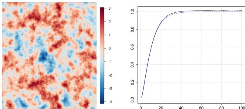
**FIG. 2 :** (Left) Simulations of a Matérn field on a 200x200 grid using Cholesky factorisation. (Right) Mean variograms over 50 simulations (solid line) and model (dotted line) : range=25, sill=1, smoothness=1.
