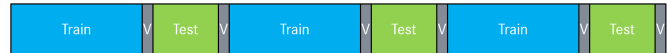
Fig. 3. The applied test, val, and train split visualized for one city. Assuming a recording length of one hour for this city, the whole session is divided into three equidistant 20 minute subsets. Each subset is then split into train, validation, and test by a 60%, 10%, 30% distribution.
