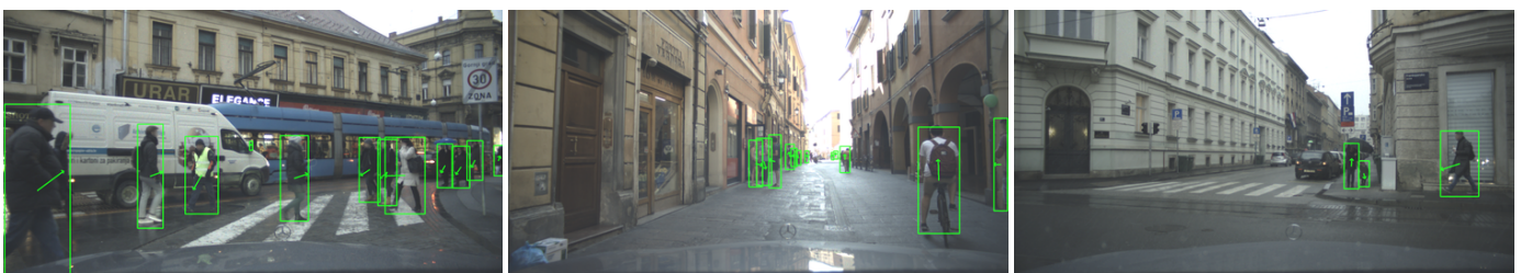
Fig. 7. Qualitative results for orientation estimation. Left and middle image show correct estimations. Right image contains a rare failure case (left person has orientation offset of about 180 degrees)
