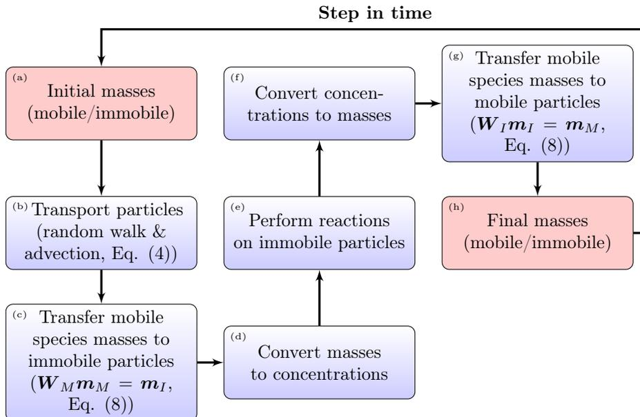
**Figure 1:** Flowchart demonstrating the order of operations for the miRPT algorithm.
