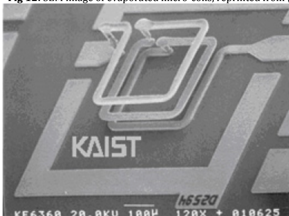
Fig 13: \mu\text{coil} monolithically obtained in CMOS technology by metal lines, SEM image from KAIST
