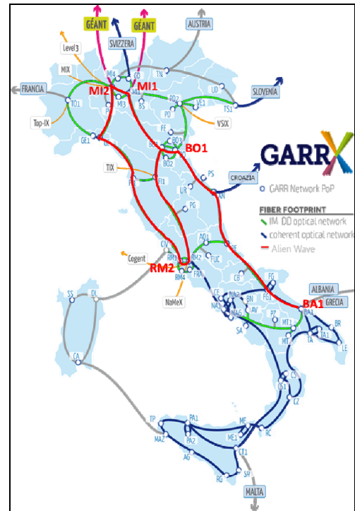
Fig. 7. GARR Alien wavelength production network deployment
