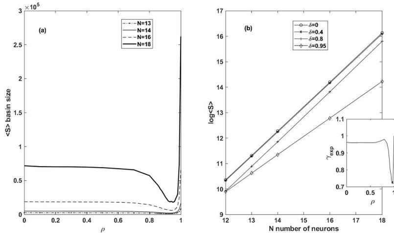
Figure 5: (a) The plot shows how the average basin size  $\langle S \rangle$  changes as a function of the dilution parameter  $\rho$  for different values of  $N$ ,  $N = 13, 14, 16, 18$ . (b) Shows how  $\langle S \rangle$  scales with  $N$  for  $\rho = 0, 0.4, 0.7, 0.95$ . The insert shows the exponential scaling coefficients for different  $\rho$  values. **This figure shows that the region with the maximum storage capacity is characterized by many small attraction basins.**
