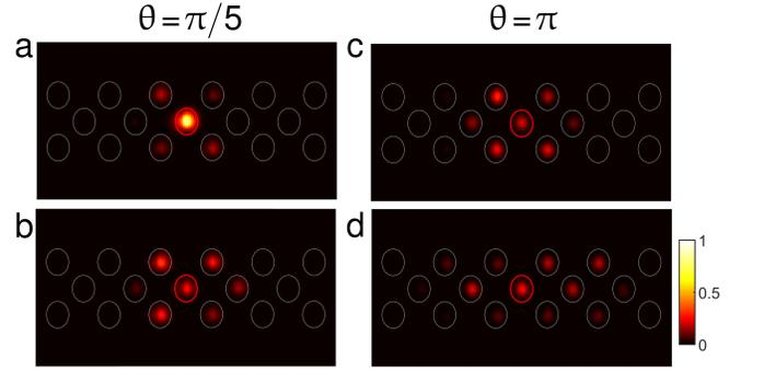
Figure A5. (a, b) Experimentally measured output intensity distributions at  $z = 35$  mm and  $70$  mm, respectively, for  $\theta = \pi/5$ . The red circled  $A$  site was initially excited for all measurements. Here,  $K/\omega = 1.35$ . (c, d) Same as (a, b) with  $\theta = \pi$ .
