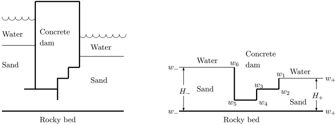
Figure 1: Left: Cross section of a rectangular dam; Right: Porous layer is a domain of the solution
