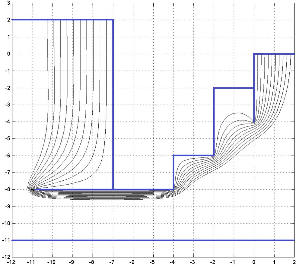
Figure 4: Global behaviour of the stream lines under the dam with additional riblets.
