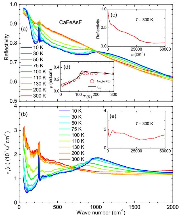
Figure 1. (color online) (a) Far-infrared reflectivity of CaFeAsF at different temperatures. Inset (c): 300-K reflectivity over a broad frequency range. Inset (d): Comparison of the *dc* resistivity,  $\rho_{ab}$  (solid line), with the zero-frequency values of the Drude fits to the conductivity data (open circles). (b) Far-infrared optical conductivity of CaFeAsF at different temperatures. Inset (e): Optical conductivity at 300 K over a broad frequency range.
