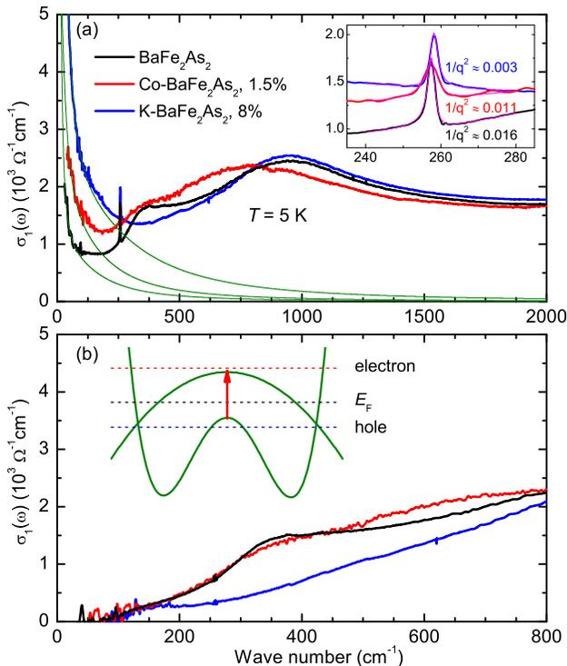
Figure 3. (color online) (a) Optical conductivity of undoped, Co (electron) and K (hole) doped  $\text{BaFe}_2\text{As}_2$  at 5 K. The inset shows the infrared-active phonon and the corresponding Fano fits. (b) The subtracted spectra in the low-energy region. The diagram shows a schematic band dispersion of a pair of Dirac cones with the same chirality [12].
