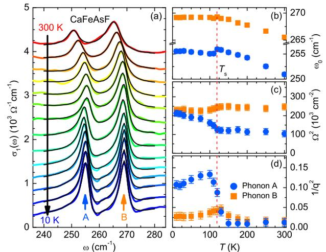
Figure 4. (color online) (a) Line shape of the infrared-active phonon modes at temperature from 300 to 10 K. The black solid lines through the data denote the Fano fits. (b–d) Temperature dependence of the resonance position  $\omega_0$ , intensity  $\Omega^2$  and Fano parameter  $1/q^2$  of the two phonons. The vertical dashed line denotes the structural transition temperature  $T_s$ .
