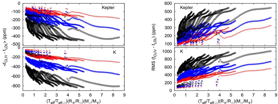
**Figure 6.** (Left) Average differences between synthetic planetary transit light curves computed using model stellar atmosphere CLIV or using best-fit quadratic limb-darkening laws as a function of atmospheric extension for the *Kepler*-band (top) and *K*-band (bottom). (Right) Same as the left panels but for the RMS difference of the light curves. The red crosses represent transits with  $\mu_0 = 1$ , blue stars  $\mu_0 = 0.7$  and black open squares  $\mu_0 = 0.3$ .
