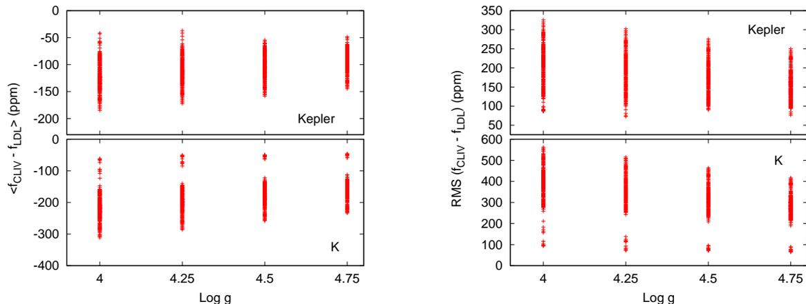
**Figure 2.** (Left) Average differences between synthetic planetary transit light curves computed using model stellar atmosphere CLIV and using best-fit quadratic limb-darkening laws as a function of stellar gravity for the *Kepler*-band (top) and *K*-band (bottom). (Right) Same as the left panels but for the RMS difference of the light curves.
