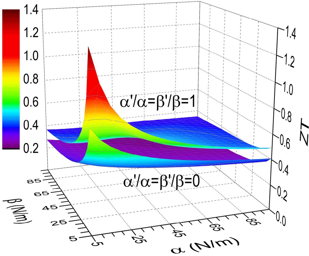
**FIG. 3.** Dimensionless thermoelectric figure of merit ( $ZT$ ) as a function of the central ( $\alpha$ ) and non-central ( $\beta$ ) restoring force constants with  $\varepsilon_0 = -0.027|t|$  for a poly(G)-poly(C) DNA chain of five GC base pairs connected to two semi-infinite atomic leads with the same parameters of FIG. 2.
