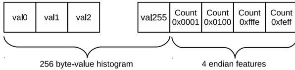
Figure 1: Layout of the full 260-dimension feature vector.
