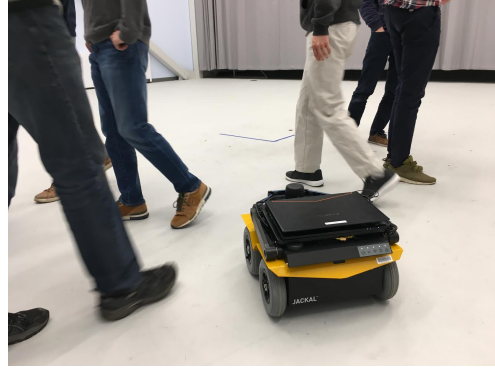
Fig. 1: A robot navigates among pedestrians. Robots use onboard sensors to perceive the environment and run collision avoidance algorithms to maintain safe and efficient operation.
