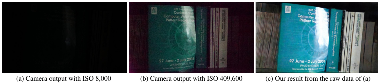
Figure 1. Extreme low-light imaging with a convolutional network. Dark indoor environment. The illuminance at the camera is < 0.1 lux. The Sony \alpha 7S II sensor is exposed for 1/30 second. (a) Image produced by the camera with ISO 8,000. (b) Image produced by the camera with ISO 409,600. The image suffers from noise and color bias. (c) Image produced by our convolutional network applied to the raw sensor data from (a).
