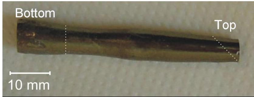
FIG. 20. The single crystal [47] of \text{Ce}(\text{Fe}_{0.76}\text{Ru}_{0.24})_2\text{Ge}_2 used for all single crystal neutron scattering experiments. The part labeled 'bottom' exhibited long-range order (see Fig. 6) and was part of the first HB3 experiments, subsequently masked with Gd paint for follow-up HB3 experiments, and cut off in later experiments (DCS, TRIAX, BT7). The part labeled 'top' was cut off and used in specific heat, susceptibility, and resistivity measurements.
