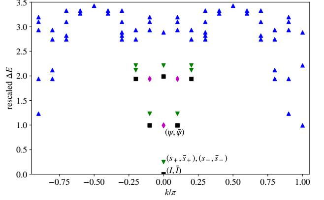
FIG. 2. The energy spectrum of the XY model with  $L = 20$ . The four primary states are marked by  $(I, \bar{I})$ ,  $(s_+, \bar{s}_+)$ ,  $(s_-, \bar{s}_-)$  and  $(\psi, \bar{\psi})$  in the spectrum. The energy differences  $\Delta E$ 's have been rescaled according to the scaling dimensions of the primary states. The states in the same conformal tower are marked by the same color with the corresponding primary state, while the unidentified states are marked as blue.
