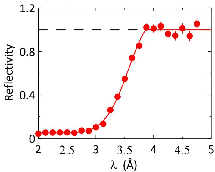
Figure 4: Reflectivity curve of the mirror collected integrating the diffracted intensity on four strips corresponding to about 0.1 degree interval. The raw data are shown.
