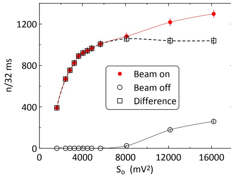
Figure 10: Results of the full pulse shape analysis. Neutron flux as a function of  $S_o$ . Red full circles, beam-on data. Black open circles, beam-off data. Black empty squares, difference between beam-on and beam-off data. The lines are guide to eyes.
