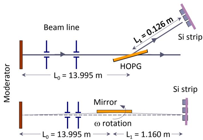
Figure 1: Schematics of the neutron measurements setup on the ALF beam line at ISIS. The upper panel refers to the HOPG crystal or the Ni polycrystal configuration while the lower panel refers to the reflectivity setup for the test on the mirror. Note the short secondary path used in both cases.
