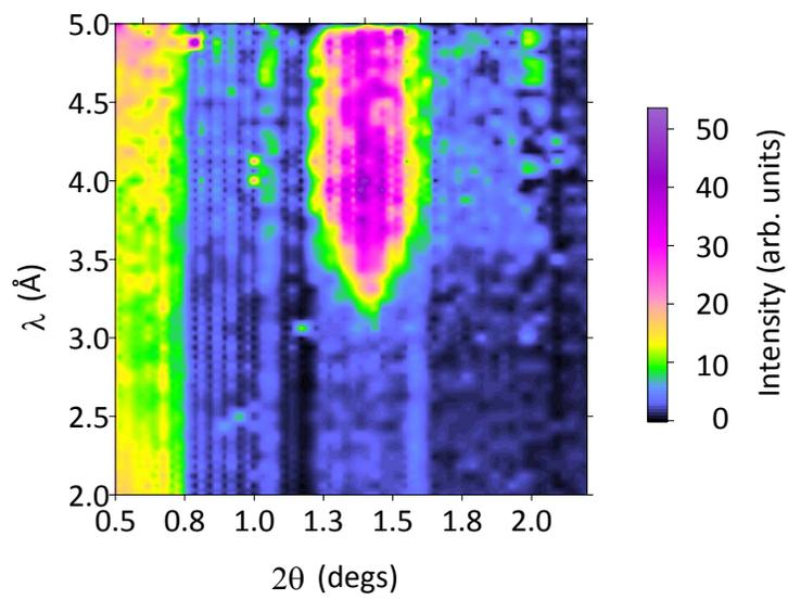
Figure 3: Intensity map diffused by the mirror located at the sample position as a function of diffraction angle at the detector and wavelength. The critical wavelength at about 3.4 Å is clearly visible.
