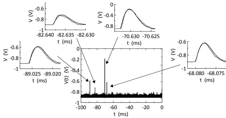
Figure 8: Typical experimental spectrum collected from a PIN diode plus  $Gd_2O_3$  converter. The signal contains four peaks identified as neutrons clearly visible above random noise. The four neutron peaks present in the signal are shown in the expanded plots (thin line) in comparison with the model fitting functions (thick line).
