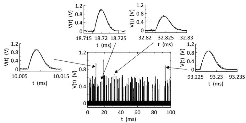
Figure 7: A typical signal produced in the simulation, lasting 100 ms, is presented. Almost all the visible peaks do not belong to a nominal neutron peak. The four neutron peaks present in the signal are shown in the expanded plots (thin line) in comparison with the model fitting curves (thick line).
