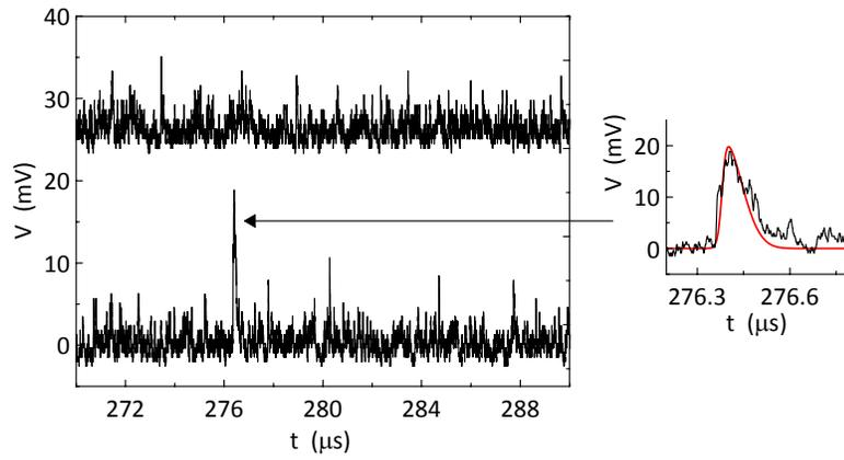
Figure 9: Typical experimental spectrum collected from the SiPM coupled to a GS20 scintillator (bottom black line). The signal, lasting 1 ms, is presented on a fraction of the total duration to enhance the presence of a peak we can attribute to neutrons signal by comparison to the beam-off spectrum (top black line). The enlarged plot on the right side shows the peak we attribute to neutrons in comparison with the fitted peak (red thick line).
