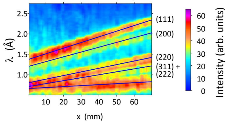
Figure 5: Intensity map of the 3 mm diameter Ni sample. The two dimensional plot does not allow for the resolution of the very short wavelength reflections below 1  $\text{\AA}$ .
