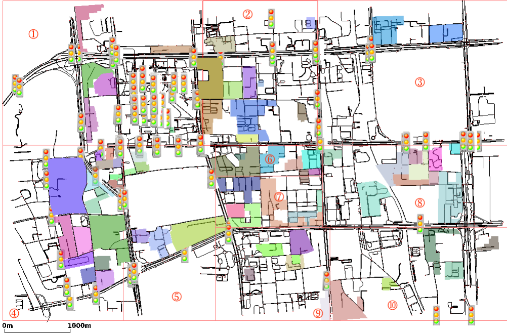
Figure 10: The Haidian-center road network. Black lines represent the roads, red points represent the intersections, colorful shadow areas represent the gated residential areas, colored lights represent the traffic lights and ten red boxes represent areas of ten projects, respectively.
