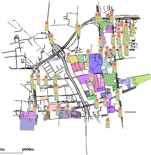
Figure 14: The Haidian-test road network. Black lines represent the roads, red points represent the intersections, colorful shadow areas represent the gated residential areas and colored lights represent the traffic lights.
