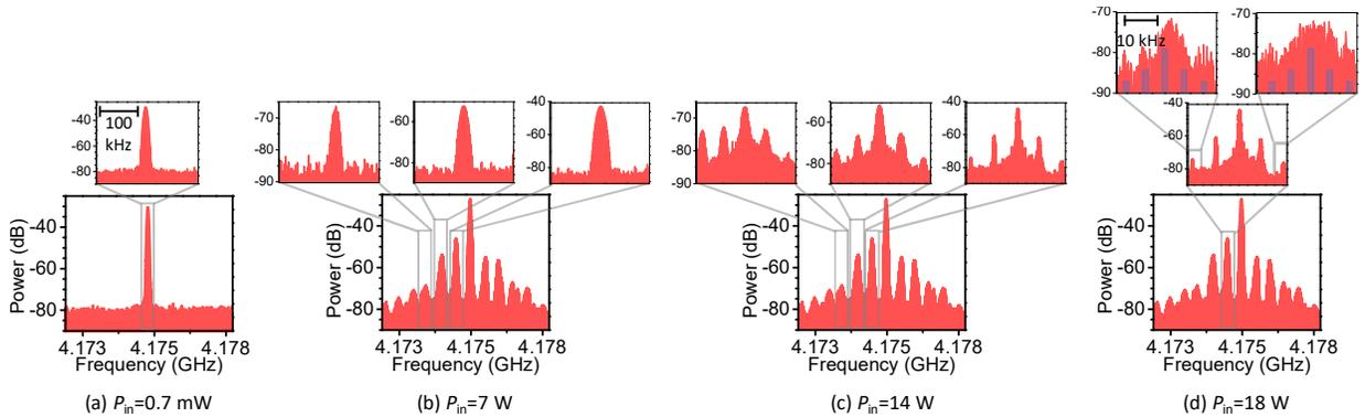
Fig. 4. Power-frequency spectra measured at different  $P_{\text{in}}$ , as indicated, demonstrating fractal development. The diagrams in the middle and top rows share the same frequency scale indicated in the left-most diagram in each row. The vertical bars in the top-row diagrams serve as visual guides to indicate the positions of the frequency peaks.
