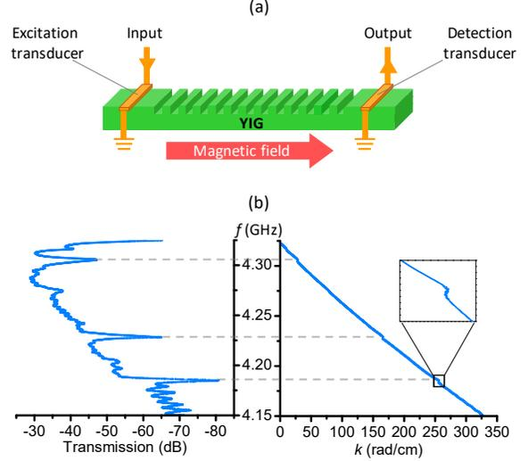
Fig. 2. (a) Experimental configuration. (b) Transmission profile (left) and frequency  $f$  vs. wavenumber  $k$  dispersion curve (right) measured with a YIG-based 1D magnonic crystal for  $P_{\text{in}}=0.7$  mW.
