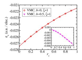
FIG. 2: (Color online) Correlation energy  $\epsilon_c$  as a function of  $r_s$  for an infinitely thin wire (and in the inset for a harmonic wire of width b = 0.5). The solid line is a quadratic fit as a function of  $r_s$ .
