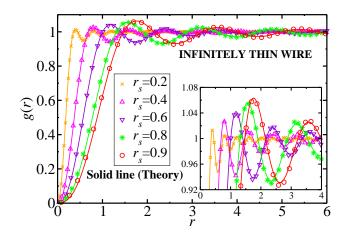
FIG. 4: (Color online) PCFs g(r) of 1D HEGs in infinitely thin wires. Results obtained from VMC simulation are compared with recent high-density theory<sup>55</sup> at several densities. The inset shows the oscillations of g(r) at larger distances in greater detail.
