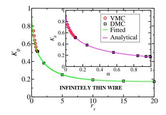
FIG. 12: (Color online) Tomonaga-Luttinger parameter  $K_{\rho}$  plotted against  $r_s$  and, in the inset, plotted as a function of exponent  $\alpha$  for an infinitely thin wire. The low density DMC data are adopted from Lee and Drummond.<sup>53</sup>
