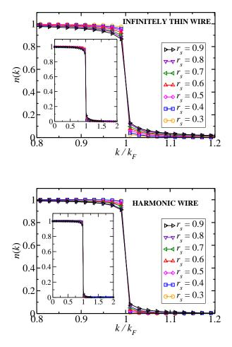
FIG. 8: (Color online) (upper) MD of an infinitely thin wire and (lower) MD of a harmonic wire of width b = 0.5 at several densities. The data shown are for N = 99. The statistical error bars are much smaller than the symbols and have therefore been omitted for clarity. The inset shows a zoomed-out view.
