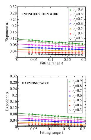
FIG. 9: (Color online) Tomonaga-Luttinger liquid exponent  $\alpha$ in Eq. (9) extracted from our MDs against the fitting range of data ( $|k - k_F| < \epsilon k_F$ ), for (upper) a ferromagnetic, infinitely thin wire and (lower) a harmonic wire of width b = 0.5 The extracted exponent is linearly fitted with the solid line in the region  $\epsilon > 0.035$  and extrapolated to  $\epsilon = 0$ .
