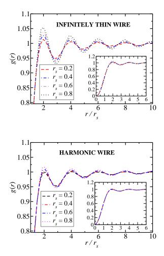
FIG. 3: (Color online) (upper) PCF of an infinitely thin wire at several densities. (lower) PCF of a harmonic wire of width b = 0.5 at several densities. The data shown are for N = 99. The inset shows the same data at the origin. The random errors in the data are small, as evidenced by the lack of visible noise in the curves.
