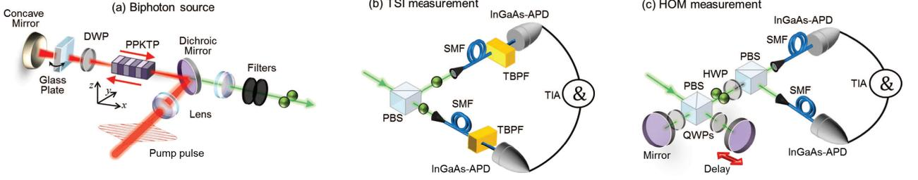
FIG. 2. Experimental setup for (a) biphoton source, (b) TSI measurement, (c) HOM measurement. DWP, dual-wavelength wave plate; SMF, single-mode fiber; APD, avalanche photodiode; PBS, polarizing beam splitter; HWP, half-wave plate.
