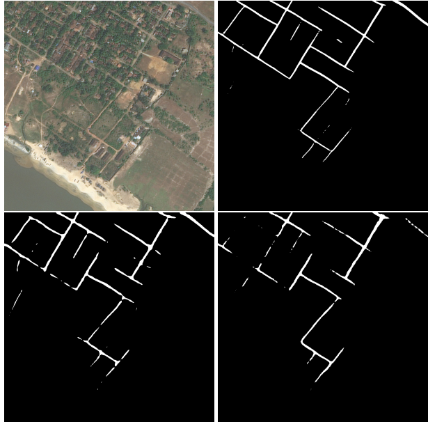
Figure 2. (Top Left) Sample image; Segmentation maps generated by ResNet50-D2S (Top Right), VGG16-BN-D2S (Bottom Left), and Segnet (Bottom Right) models, respectively.
