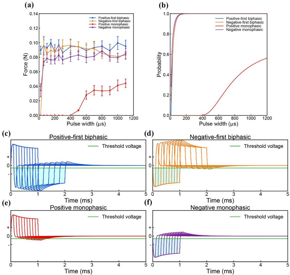
Figure S6.3.1.3 Four waveform comparison test of TA muscle stimulation with 500  $\mu\text{A}$  current amplitude. (a) Force mapping data; (b) Probability mapping result; (c) Voltage waveform of positive-first biphasic square waveform current; (d) Voltage waveform of negative-first biphasic square waveform current; (e) Voltage waveform of positive monophasic square waveform current; (f) Voltage waveform of negative monophasic square waveform current;
