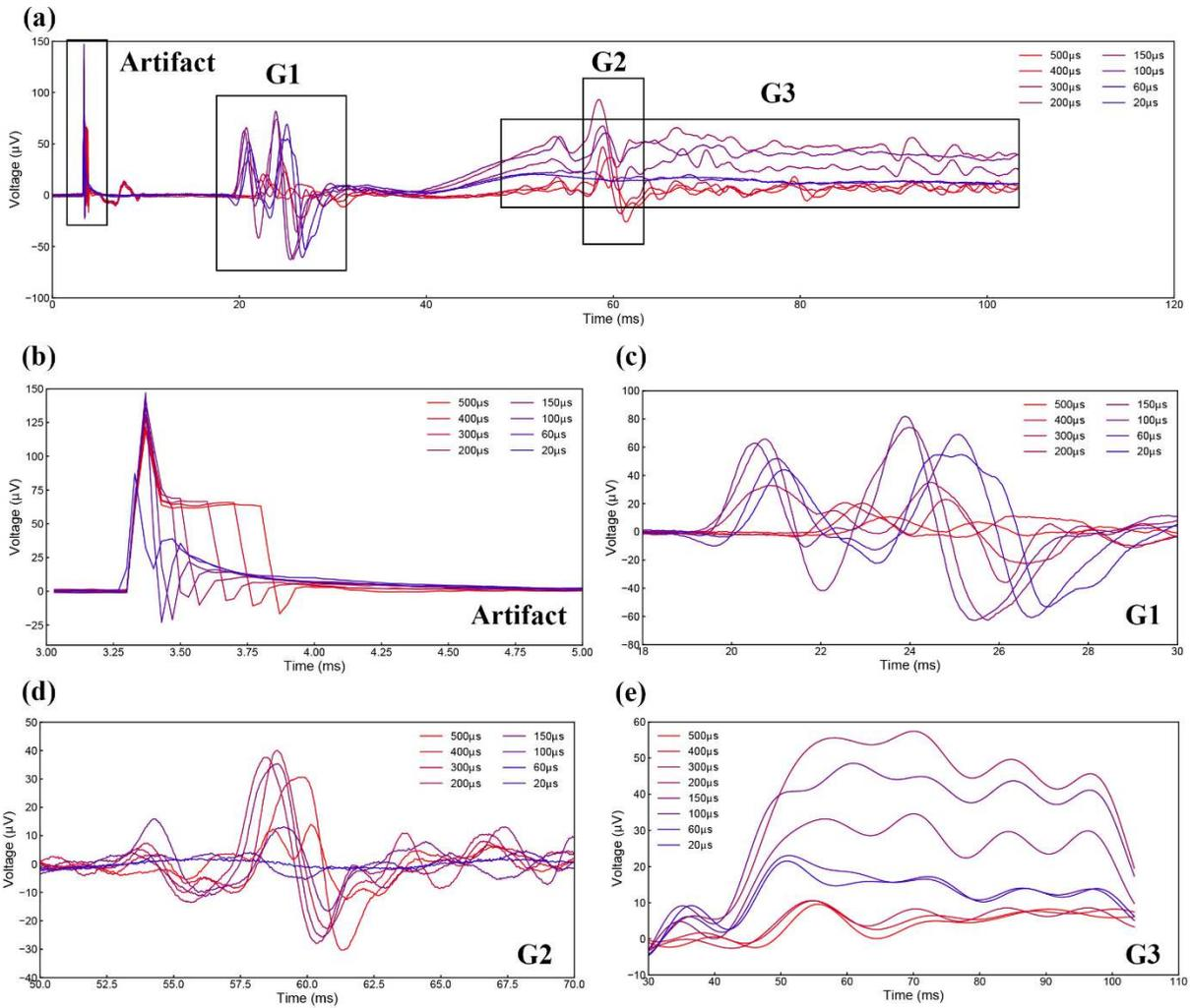
Figure S6.6.2.2 (a) Complete EMG recording result of pelvic nerve stimulation by negative monophasic square waveform current. The Current amplitude is  $70 \mu\text{A}$ ; (b) Stimulus artifact; (c) EMG signal of group G1; (d) EMG signal of group G2 by applying 80 Hz high pass filter; (e) EMG signal of group G3 by applying 80 Hz low pass filter.
