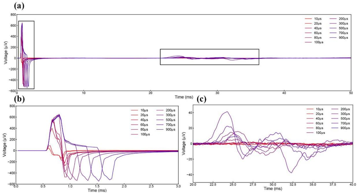
Figure S6.5.3.2 Complete EMG data of cortical stimulations with negative monophasic current waveform of 500  $\mu\text{A}$ ; (a) The complete raw EMG data; (b) The stimulus artifacts; (c) the EMG signal.
