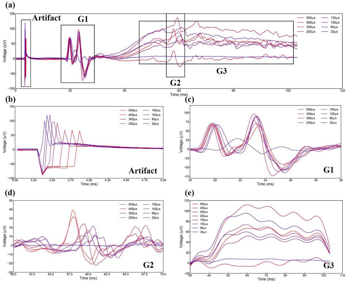
Figure S6.6.2.1 (a) Complete EMG recording result of pelvic nerve stimulation by using positive monophasic square waveform current. The current amplitude is  $70 \mu\text{A}$ ; (b) Stimulus artifact; (c) EMG signal of group G1; (d) EMG signal of group G2 by applying 80 Hz high pass filter; (e) EMG signal of group G3 by applying 80 Hz low pass filter.
