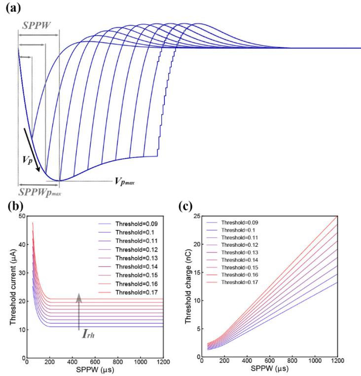
FIG. 3. Derivation of the Strength–duration relationship. (a) Illustrative voltage waveforms generated by negative monophasic square waveform current; (b) The threshold current amplitude ( $I_{th}$ ) decreases as the  $SPPW$  increases in a nonlinear fashion; (c) The relationship between threshold charge ( $Q_{th}$ ) and  $SPPW$  is linear.
