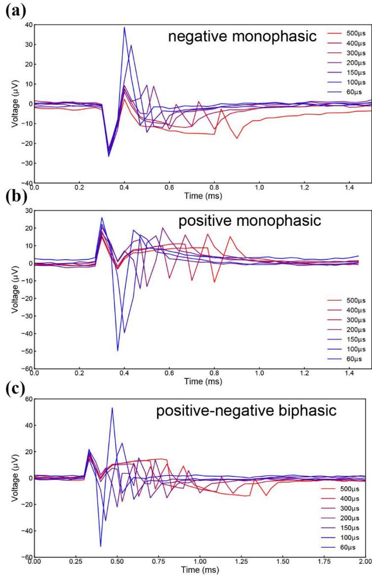
Figure S6.2.3. Stimulus artifact of pelvic stimulation with different current waveform of 70  $\mu\text{A}$ ; (a) Positive monophasic square waveform; (b) Negative monophasic square waveform; (c) Positive-first biphasic square waveform.
