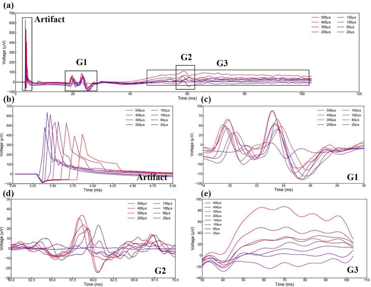
Figure S6.6.2.3 (a) Complete EMG recording result of pelvic nerve stimulation by positive-first biphasic square waveform current. The Current amplitude is  $70 \mu\text{A}$ ; (b) Stimulus artifact; (c) EMG signal of group G1; (d) EMG signal of group G2 by applying 80 Hz high pass filter; (e) EMG signal of group G3 by applying 80 Hz low pass filter.
