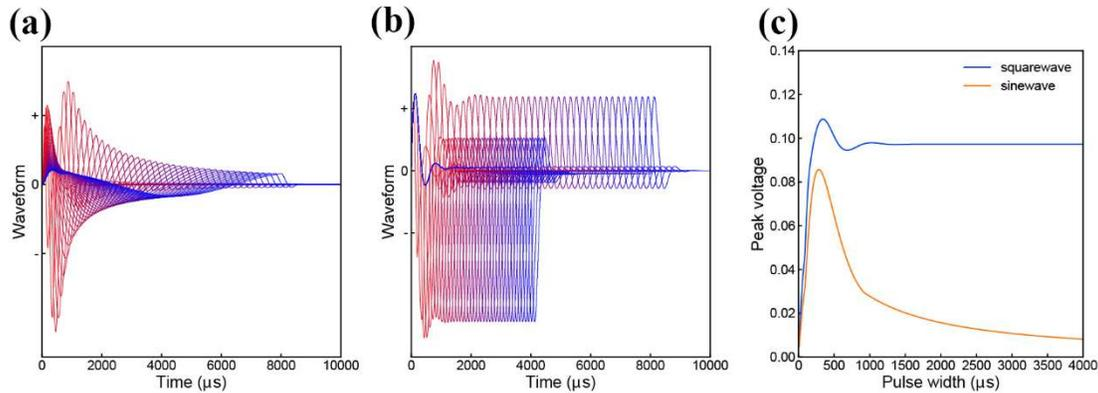
Figure S7.5 Waveform comparison of sinewave and square wave current. (a) An illustrative sinewave current with different SPPW; (b) An illustrative positive-first square waveform current with different SPPW; (c) Peak value comparison of the voltage waveform of sinewave and positive-first square wave with different SPPW.
