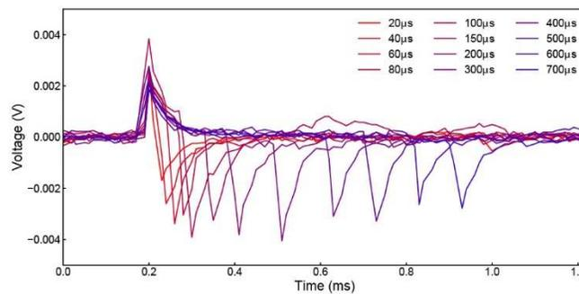
Figure S6.2.2.4. High sampling rate system (70 kHz) recording of stimulus artifact of cortical stimulation with negative monophasic waveform current of 100  $\mu\text{A}$ . The SPPW is from 20  $\mu\text{s}$  to 700  $\mu\text{s}$ .
