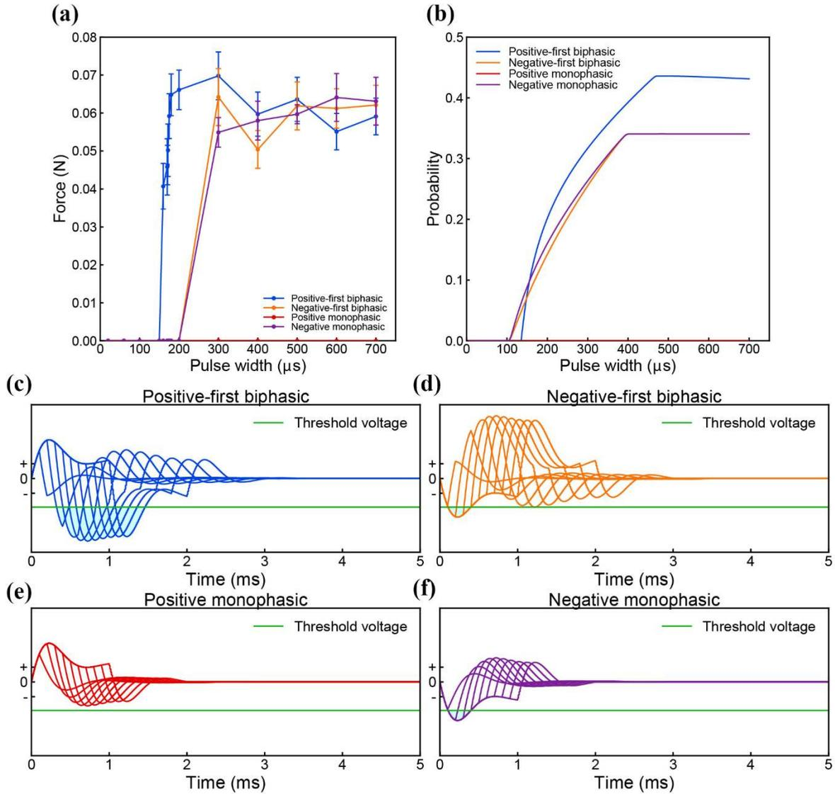
Figure S6.3.1.2 Four waveform comparison test of TA muscle stimulation with 520  $\mu\text{A}$  current amplitude. (a) Force mapping data; (b) Probability mapping result; (c) Voltage waveform of positive-first biphasic square waveform current; (d) Voltage waveform of negative-first biphasic square waveform current; (e) Voltage waveform of positive monophasic square waveform current; (f) Voltage waveform of negative monophasic square waveform current;
