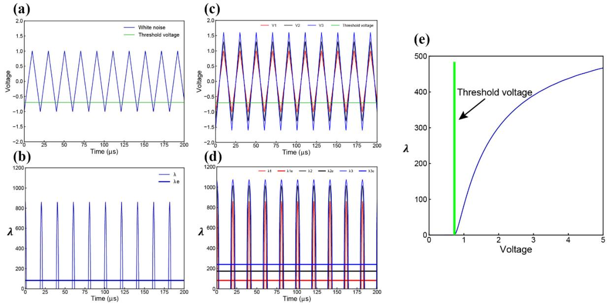
FIG. 5. Derivation of LNP model from C-P theory. (a) A simplified white noise voltage waveform; (b) The corresponding  $\lambda$  curve of the voltage waveform in (a), this  $\lambda$  curve can be averaged to a  $\lambda_e$  curve; (c) Noise with increasing amplitude; (d) The corresponding  $\lambda$  and  $\lambda_e$  curves of the noise waveforms in (c); (e) The nonlinear curve of  $\lambda_e$  versus the noise amplitude  $V_w$ .
