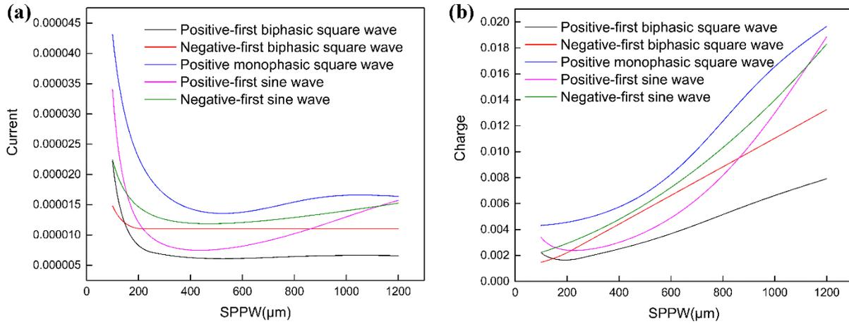
FIG. 4. (a) The relationship between the threshold current amplitude ( $I_{th}$ ) and the *SPPW* for different current waveforms; (b) The relationship between threshold charge ( $Q_{th}$ ) and *SPPW* for different current waveforms.
