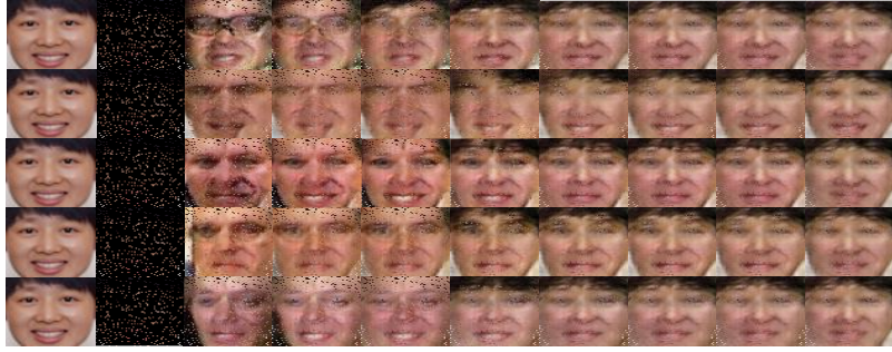
FIGURE 10. Multiple stego images generated for a single image. In each row, column 1 shows ground-truth image, column 2 shows corrupted stego images with random missing regions comprising 90% of the image, and columns 3–10 show samples generated as the number of iterations increases.
