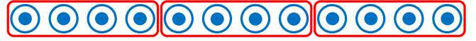
FIG. 2. Example of clustering of spins. Blue circles are physical spins \frac{1}{2} , while red rectangles are the clusters. Hamiltonian dynamics within each cluster is exact, while interactions between clusters are treated approximately.
