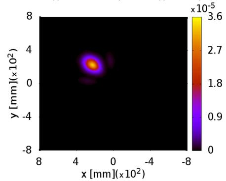
FIG. 4: (Color online) Creation of a single spot using a shifted  $HG_{11}$  control beam after propagation of  $z = 0.5 \text{ mm}$ . Other parameters are same as in Fig.(2).
