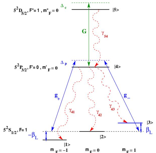
FIG. 1: (Color online) Schematic diagram of the inverted-Y level system of  $^{87}\text{Rb}$  atoms. A strong control field with Rabi frequency  $G$  couples the transition  $|4\rangle \leftrightarrow |5\rangle$ . The transitions  $|4\rangle \leftrightarrow |1\rangle$  and  $|4\rangle \leftrightarrow |3\rangle$  are coupled by the probe field components with Rabi frequency  $g_+$  and  $g_-$ , respectively
