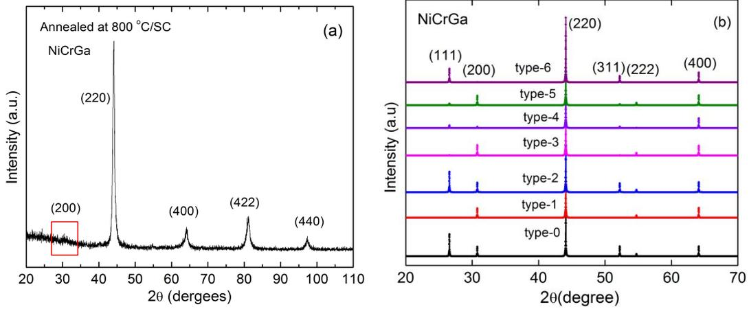
**Figure 1:** (a) Room temperature XRD patterns of NiCrGa annealed at 800°C followed by slow cooling (SC). (b) Simulated XRD patterns of NCG using Cu  $ka$  x-ray energy and the experimental lattice parameters (5.8 Å) for different types of disorders.
