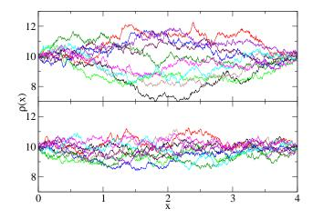
Figure 5. Particle concentration vs. position for temporal averages  $T_{\rm meas}=10^3$  in the steady state. Top:  $q\phi=0$ ; bottom  $q\phi=8k_BT$ .
