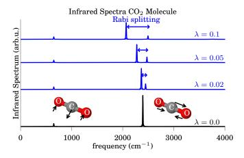
FIG. 2. Infrared spectra in vibrational strong coupling for  $CO_2$ . Black spectrum refers to the spectrum outside the cavity. We explicitly depict the two infrared-active vibrational modes of the  $CO_2$  molecule. Blue spectra correspond to the electron-nuclear spectrum. Importantly, we capture the Rabi splitting between the lower and upper polariton branch.
