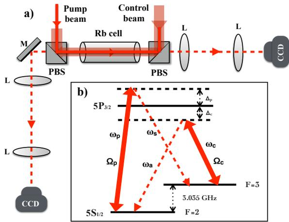
FIG. 1. a) Experimental setup for MOPO in thermal rubidium vapor, PBS: polarising beam splitter, M: mirror, L: Lens. b) Energy level diagram of  $^{85}\text{Rb}$  showing the coupling of pump and control laser fields (solid lines) and the generated Stokes and anti-Stokes fields (dashed lines).
