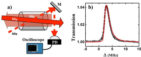
FIG. 7. a) Schematic of the experimental setup for probe propagation in N-type system. b) Matching of experimentally measured and theoretically evaluated transmission of the external probe. The black circles represent the experimental data and the red solid line represent the data from the theoretical model.
