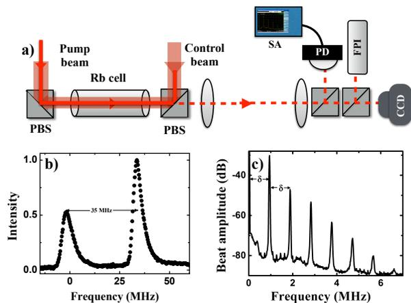
FIG. 5. Schematic of the experimental setup. b) Cavity signal showing the frequency difference of about 35 MHz between the pump and the Stokes beam using a Fabry-Perot cavity of free spectral range of 1 GHz. c) Spectrum analyzer signal showing the frequency comb under multi-spatial-mode regime.
