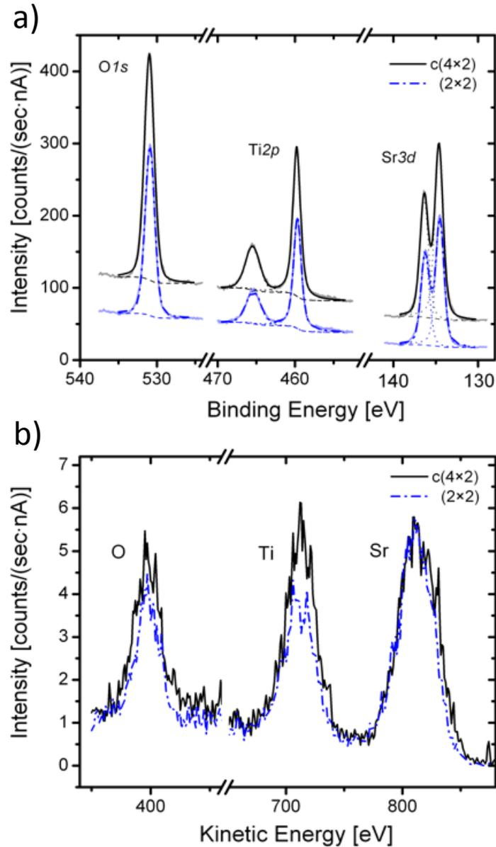
Figure 2: (a) XPS spectra (Mg K $\alpha$  with  $h\nu=1254$  eV, normal emission) and (b) LEIS spectra (averaged over 10 scans) (He $^+$  with 1 keV, scattering angle  $\theta=137^\circ$ ) of SrTiO<sub>3</sub>(001) (2x2) and c(4x2) reconstructed surfaces. The Sr to Ti peak intensity ratios are listed in Table 1.
