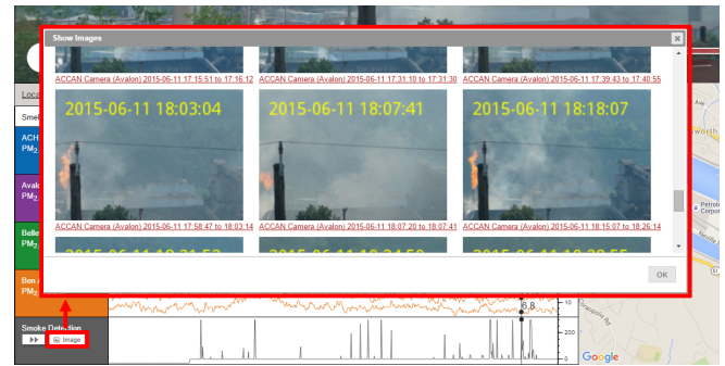
Figure 4. Clicking the image button on the line charts on the main user interface (see Figure 2) shows web links and animated images produced by the smoke detection algorithm. Users can quickly select representative images and insert them into an online document. Users can also click on a peak of a spike on the line chart to seek to a video frame with fugitive emissions.
