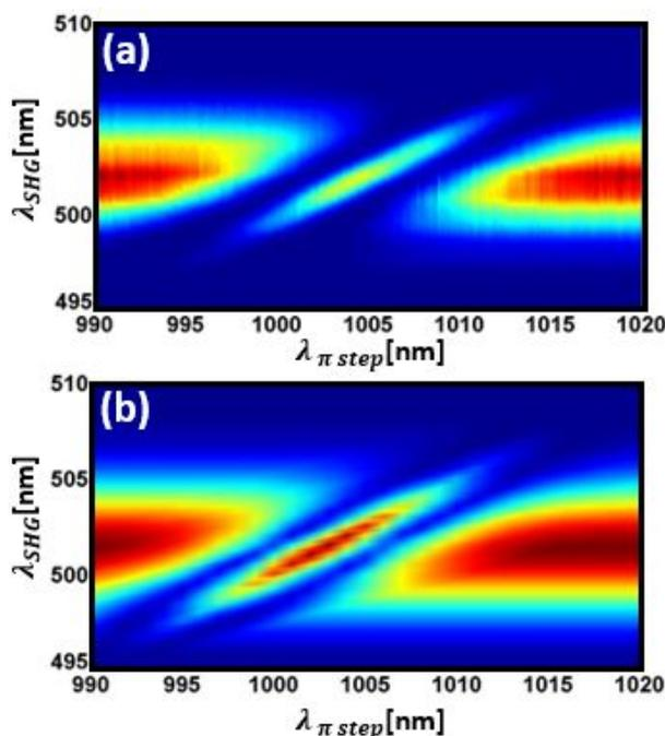
Fig.4: ASHG conversion in KTP crystal excited by a pulse with a spectral phase of  $\pi$ -step, as a function of the step position. (a) Experimental results. (b) Simulation results. The simulation results were obtained by inserting the measured spectrum of the original pulse.
