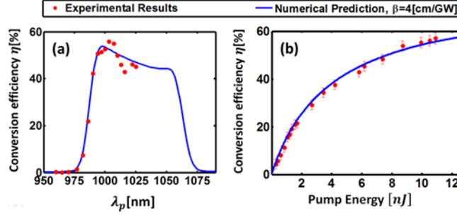
Fig. 2: Frequency conversion dependence with pump central wavelength and energy. (a) Conversion efficiency dependence with pump central wavelength. (b) Conversion efficiency as a function of pump energy centered at 1005nm wavelength. Deviation between the loss-free numerical prediction [23] and new experimental results can be attributed to TPA.
